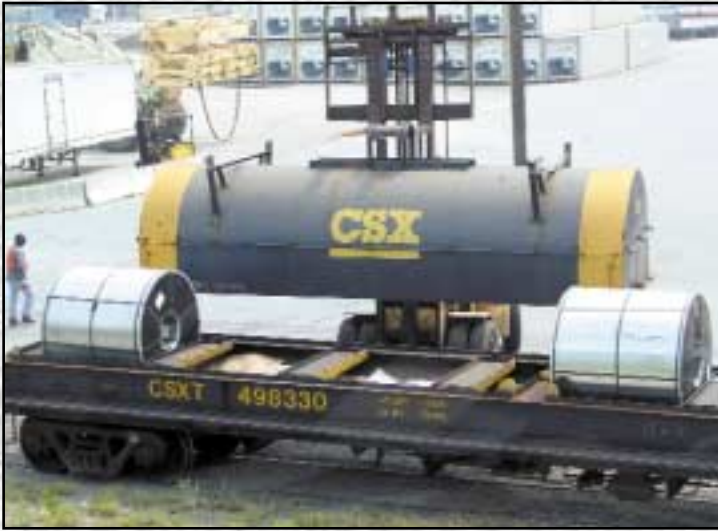
Cold rolled steel coils loaded into coil cars for a major steel mill in Pennsylvania.
