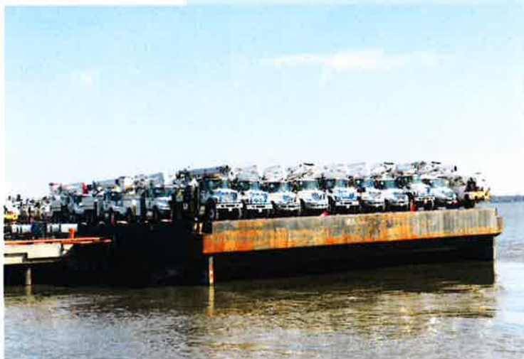
Utility vehicles were fastened to the barge using "D" rings and lashings to keep them from shifting during the voyage.
