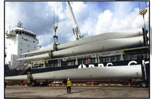
50.2 m wind turbine blades safely transferred on stretched-trailers to storage
