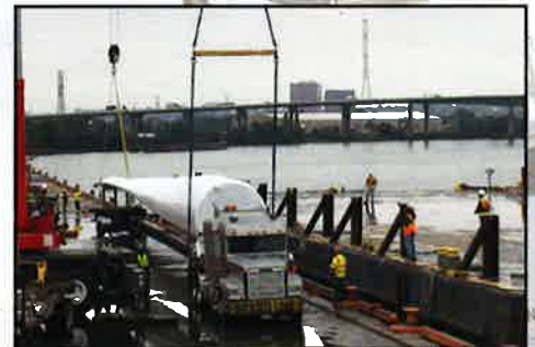
Loading 56.9 m Test Blade onto Barge
