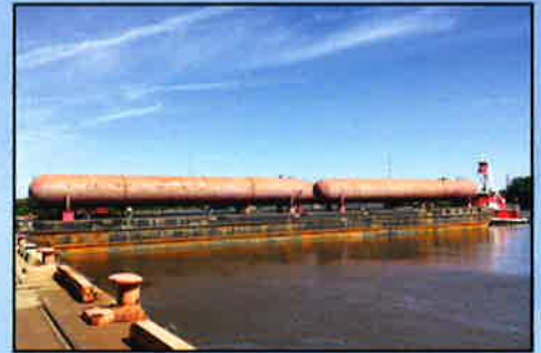
CO2 STORAGE TANKS - 120 ft long & 100 tons from barge.
